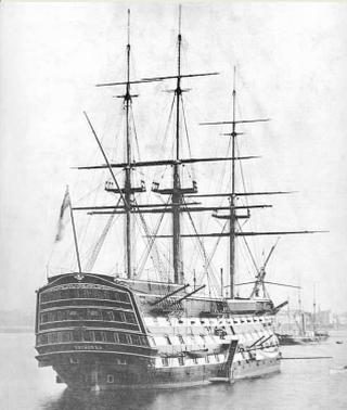
In the British Royal Navy, a **second rate** was a ship of the line which by the start of the 18th century mounted 90 to 98 guns on three gun decks; earlier 17th-century second rates had fewer guns and were originally two-deckers or had only partially armed third gun decks. The term in no way implied that they were of inferior quality. They were essentially smaller and hence cheaper versions of the three-decker first rates. Like the first
